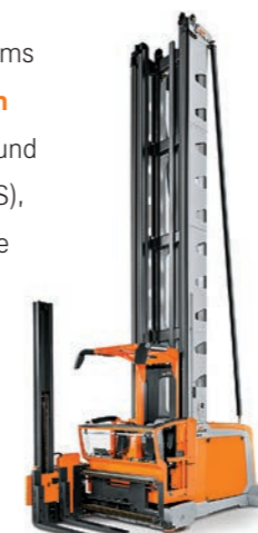
NXV The very narrow aisle truck is the ideal partner for efficient use of space in small warehouses. Optional positioning aids, such as the cross-line laser between the forks or camera systems, help you to position the load accurately.
