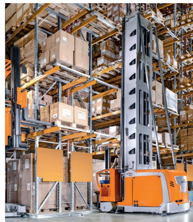
MX-X With state-of-the-art assistance systems such as Active Floor Compensation (AFC) to compensate for uneven ground and the Active Load Stabilisation (ALS), the MX-X offers ultimate performance and safety in narrow aisles.
